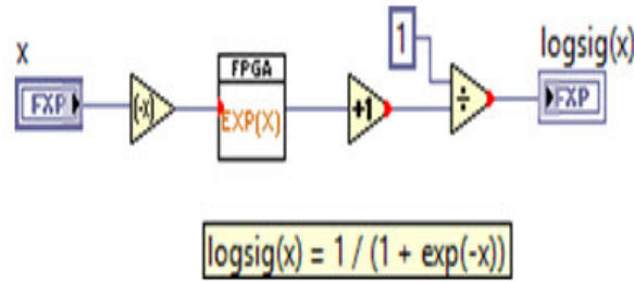
Figure 10: Logsig activation function constructed in FPGA
