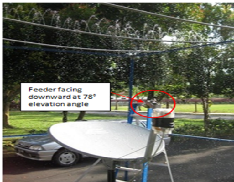
Figure 7: Feeder facing downward at 78° Elevation Angle
